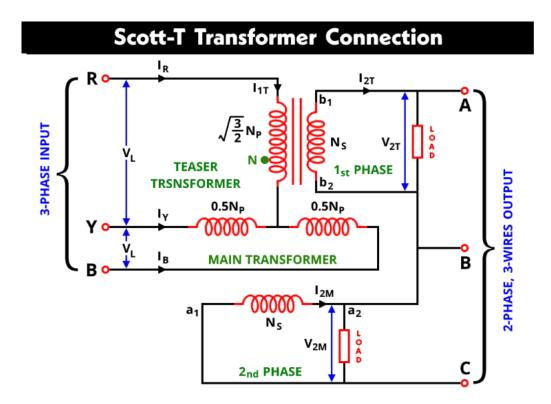
The Scott connection can be visualized through the following diagram: In the diagram:
